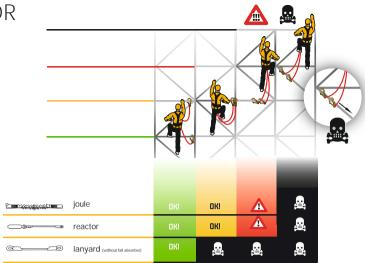
When safeguarding an ascent using a fall arrest type  $_*Y^*$  it is necessary to move at the level FF1 and lower. It means that the connectors (EN362) connected to the fall absorber (EN355) during the ascent do not  $_*$ fall  $_*$  below the connection point of the harness (EN361) in which the absorber is connected to the harness.
