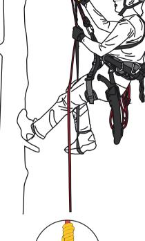
There are several methods of how to use rope techniques to get from the ground into a tree. One method is using a footlock.
