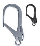
with double trigger automatic locking ga te opening 110mm • 25 kN polished, A I • 965g • 34.04 oz unique production number 0321 • EN 362
